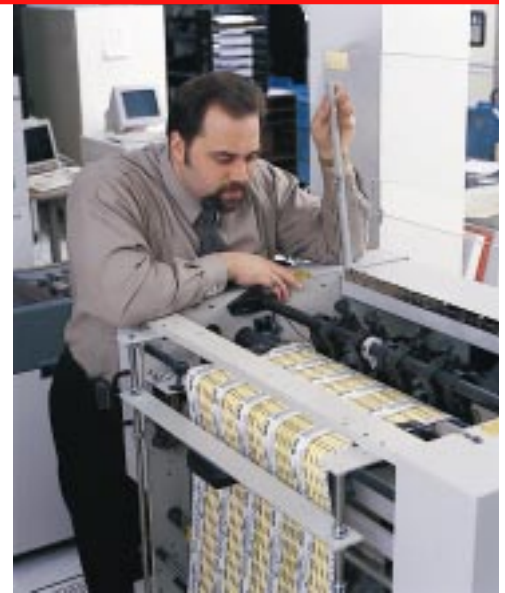
Mark Milam, Consolidated Information systems operations supervisor, watches the labels pass through the versatile slitting mechanism. The sheet is slit five labels wide – once along each white portion – and refolded into individual stacks.
