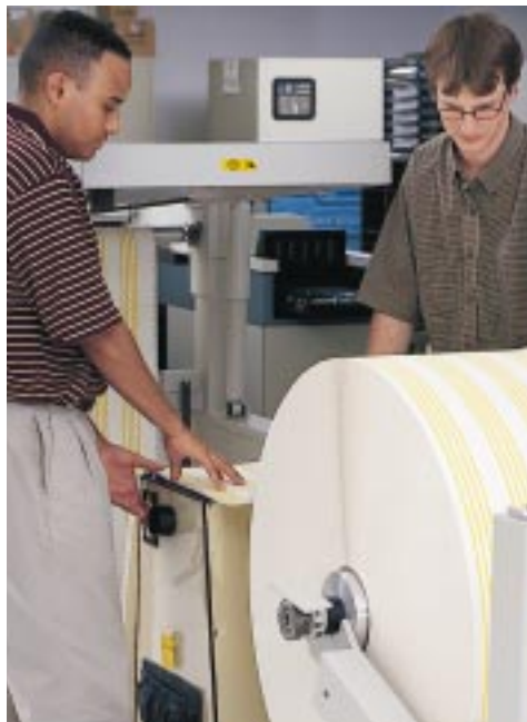
Joey Curtis (left) and Marc Poland, Consolidated computer operators, splice a new 40-inch label roll onto the end of a current roll for continued printing. Consolidated prints 283 rolls annually.
